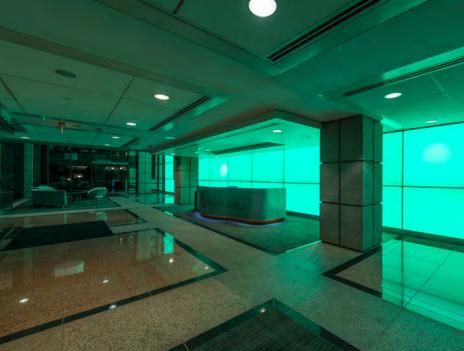
Note: The LED light boxes, utilized in the design, were created in-house in order to show the most even amount of light and color, while using the least amount of LED lights to conserve energy and emitting less heat.
